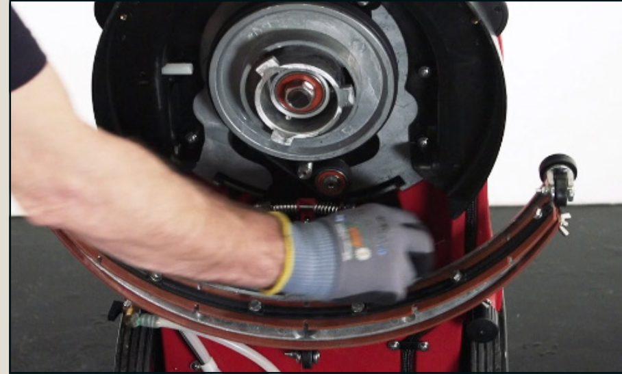
Take the squeegee off, check and clean the blades
